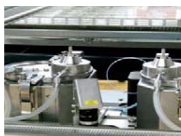
Variable y-axis the distance between solder nozzles is adjustable between 80 and 200 mm, providing an efficient method to process panels
