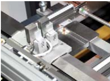
Precision spray fluxer with integrated spray stream control
