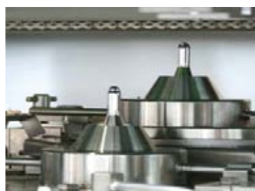
Variable z-axis on solder bath
