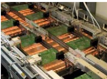
segmented short wave emitter cassette
