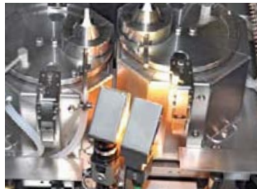
Alternatively to the single wave pot, multi wave pots are also available
