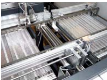
Lower preheater with short wave IR emitters
