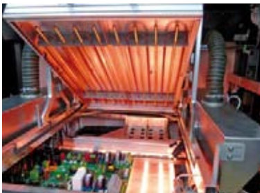
Ersselective preheat concept a perfect combination of dynamic lower and upper venturi induced convection preheater for reproducible results
