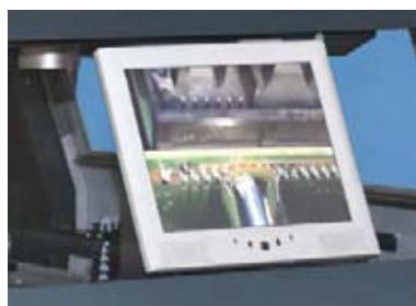
Visual process control; An optional camera system depicts the soldering results
