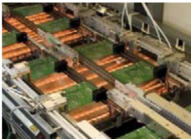
Dual conveyor doubles the throughput without increasing floorspace
